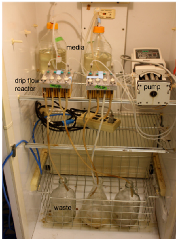
Figure 1. The drip flow reactor setup. Important components are labeled.
