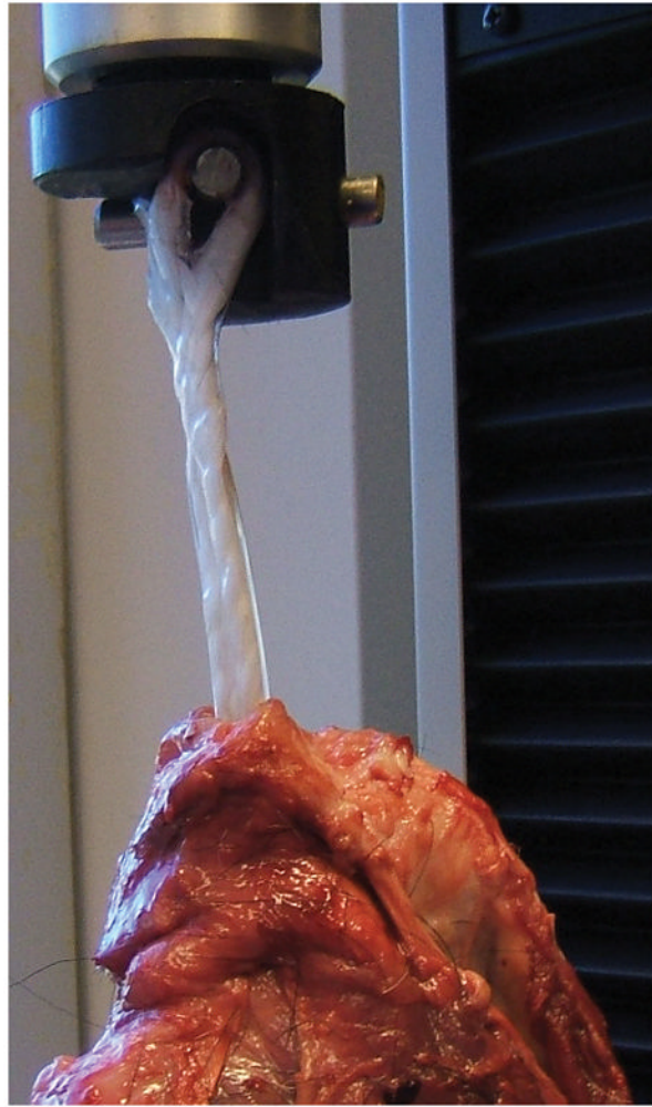
Figure 3. Explanted device on mechanical test platform. The silicone-impregnated strap (the exposed mobile portion of the device, which slides in the trochlear groove) remained free of adhesions.
