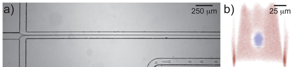
FIG. 4. (a) Without forcing, threads of dextran in PEG are stable over significant lengths, which exceed the theoretically predicted break up lengths by an order of magnitude. Droplets are visible in the bottom right of the micrograph as the channel meanders as indicated in Fig. 2. (b) Cross sectional view of the channel taken 2 mm downstream of the cross junction showing that the thread is centered and does not touch the walls.
