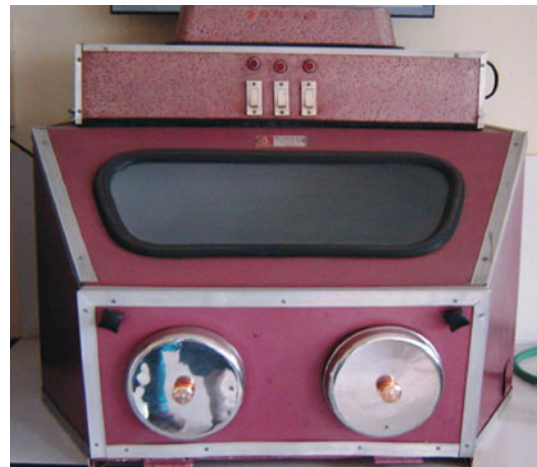
Fig. 2 UV light disinfection unit
