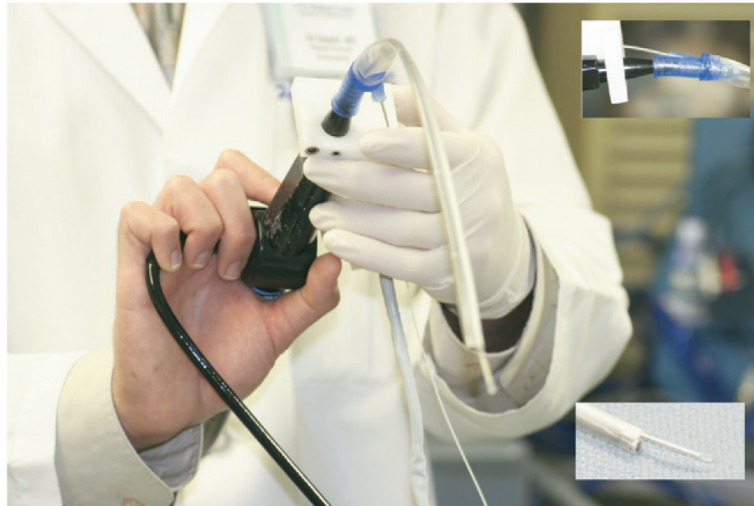
Figure 3. The slide-on channeled endosheath through which the rhinolaryngoscope and OCT probe were placed ( top right inset ) and coupled at their distal ends ( bottom right inset ).
