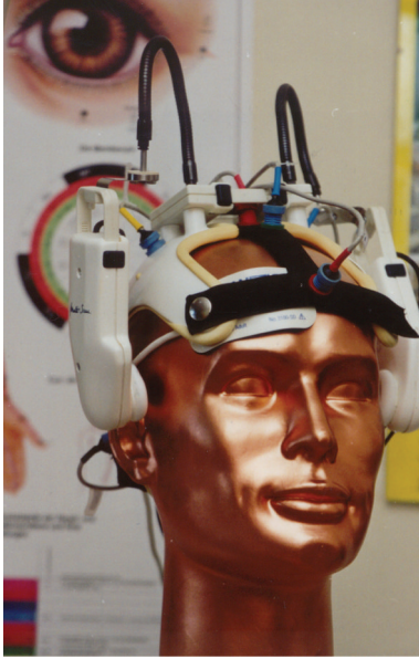
FIGURE 17: Helmet construction from our research group for the first proof of changes in blood flow velocity in the brain caused by acupuncture. Modified from [45].
