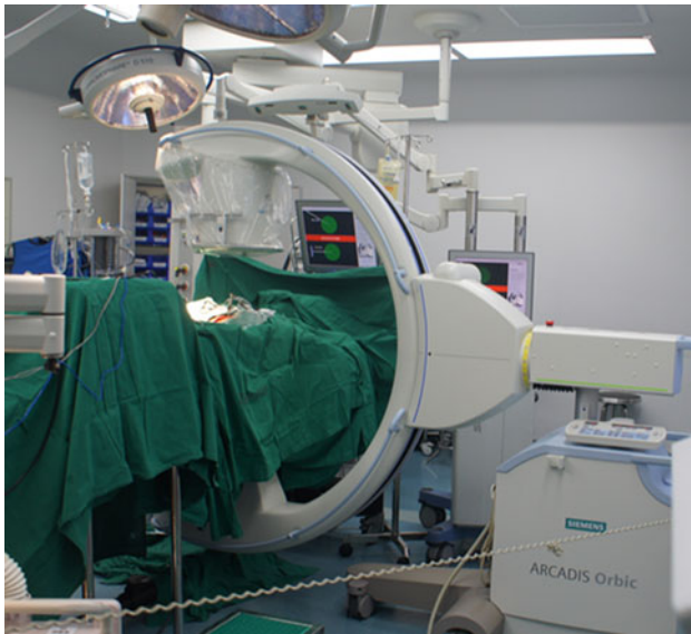
Fig. 1 Operative setup of the intraoperative 3D fluoroscopy-based navigation system with the computer screen facing the surgeon
