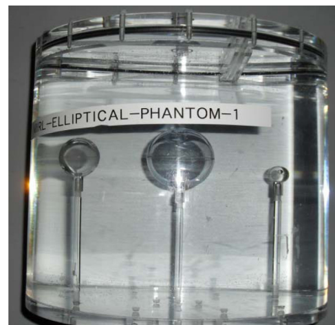
Fig. 5. Elliptical phantom used in physical phantom experiments showing three spheres of different sizes.
