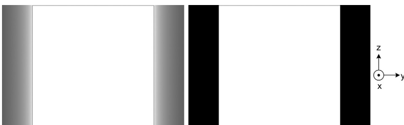
Fig. 15. Representative slice of the completeness map for an inverse-geometry scan mode with source size 231.2 \times 160 mm and the detector size W \times H = 50 \times 160 mm. While the left image is in a display window of [0, 1] , the right image is the indicator of exact reconstruction region. The square boxes indicate the VOI, which is covered by the exact reconstruction region.
