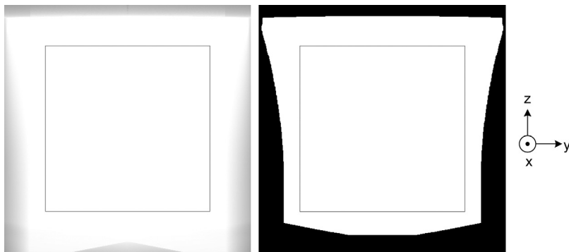
Fig. 16. Representative slice of the completeness map for a composite-circling scan mode with R_1 = 100 mm, planar detector W \times H = 536.3 \times 637.6 mm. While the left image is in a display window of [0, 1] , the right image is the indicator of exact reconstruction region. The square boxes indicate the VOI, which is covered by the exact reconstruction region.
