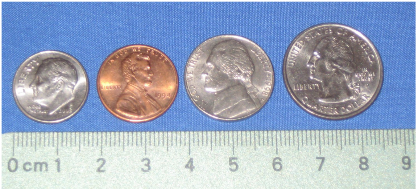
Figure 2. United States coins by size. Standard U.S. Mint coin diameters are 17.91 mm for a dime, 19.05 mm for a penny, 21.21 mm for a nickel, and 24.26mm for a quarter.
