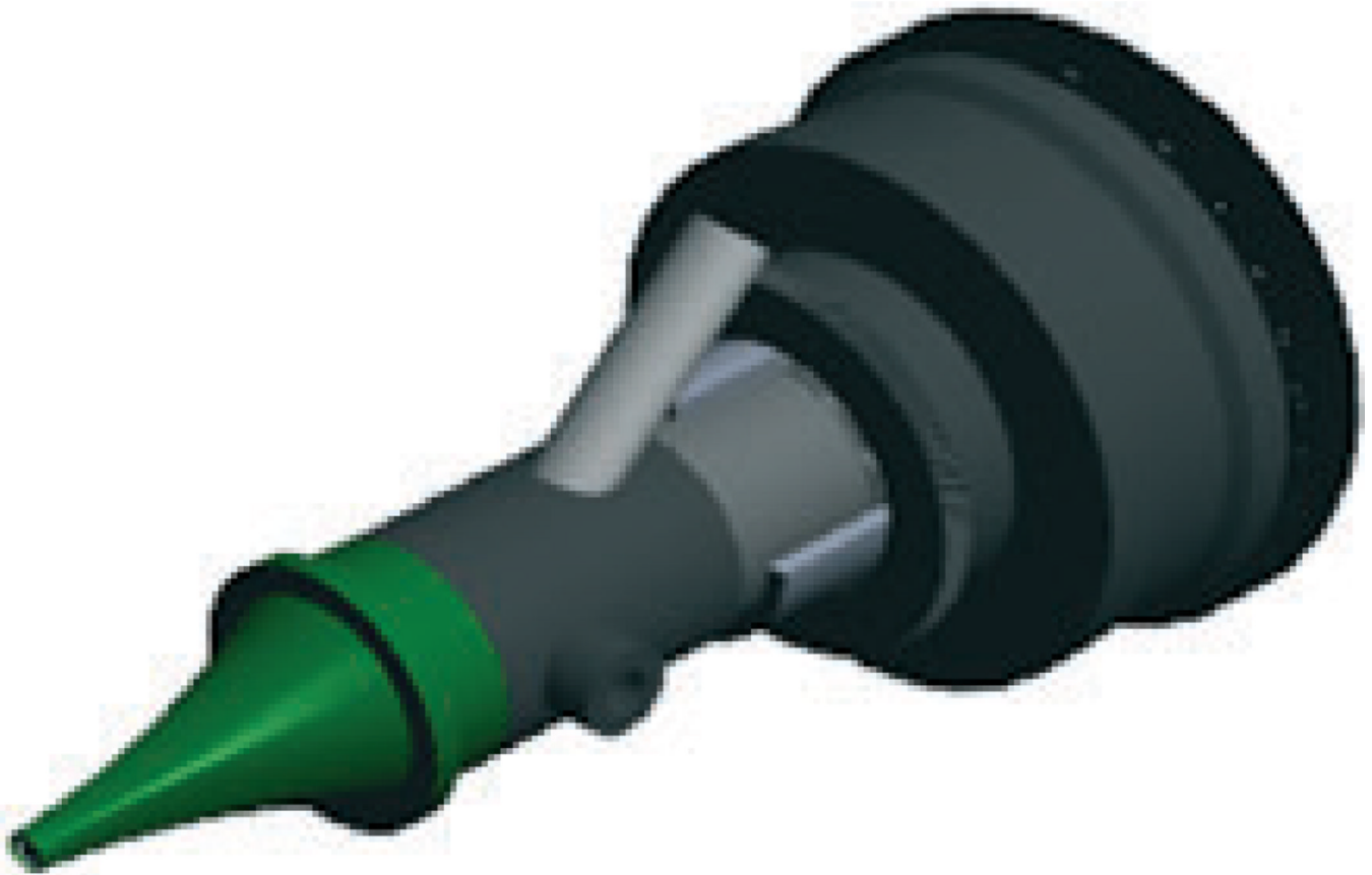
Figure 2. Computer-Aided Design of the optical section of the Rol gradient-index fundus imaging system.
