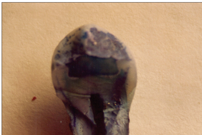
Figure 5: Ormocer: An aesthetic direct restorative material. Linear dye penetration in Group V – positive control, Mean – 1.500 mm
