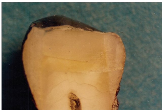
Figure 4: Ormocer: An aesthetic direct restorative material. Linear dye penetration in Group IV – Admira with Admira Bond, Mean – 0.200 mm
