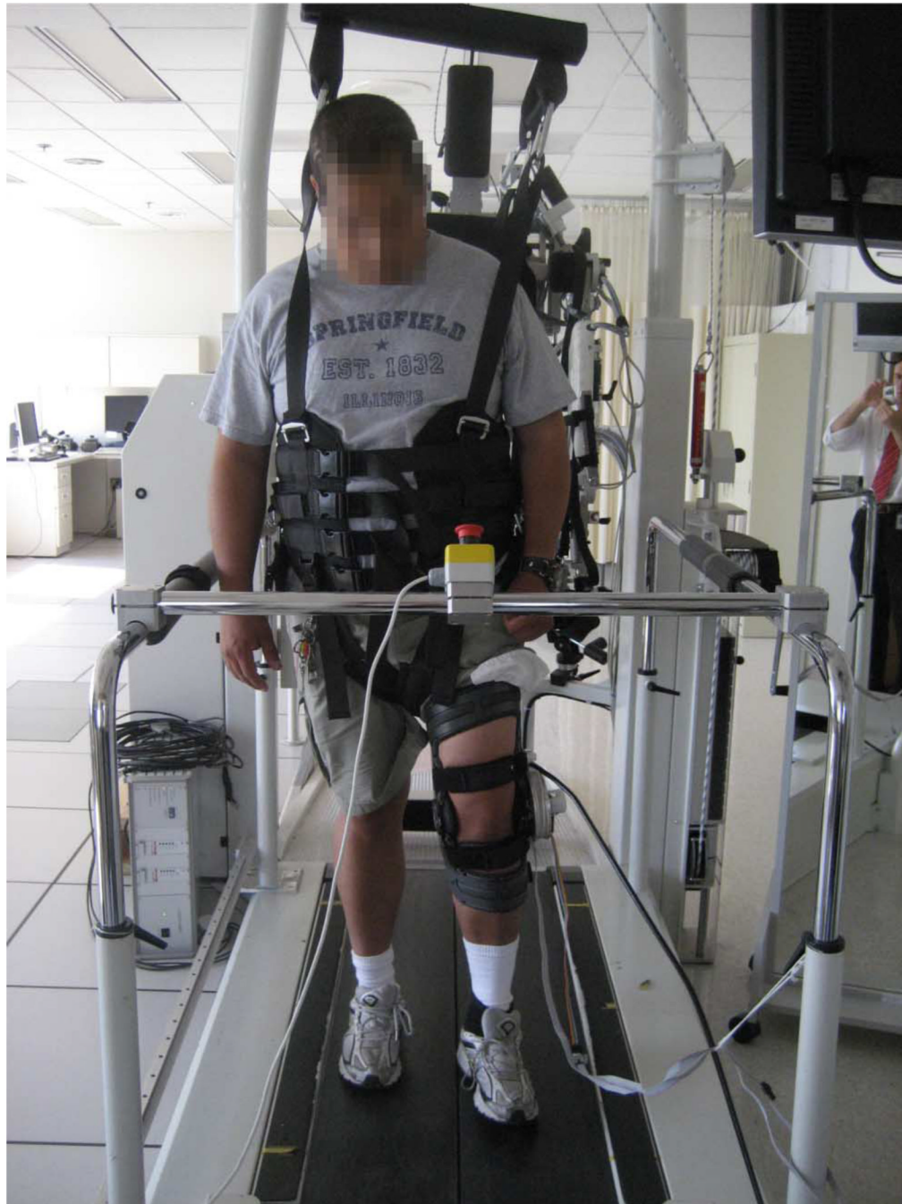
Fig. 5. Experimental setup where a subject wears a harness to be protected from falls. Cables leading to device are for Bowden actuation and sensors, whose weight is partially supported at the bar.
