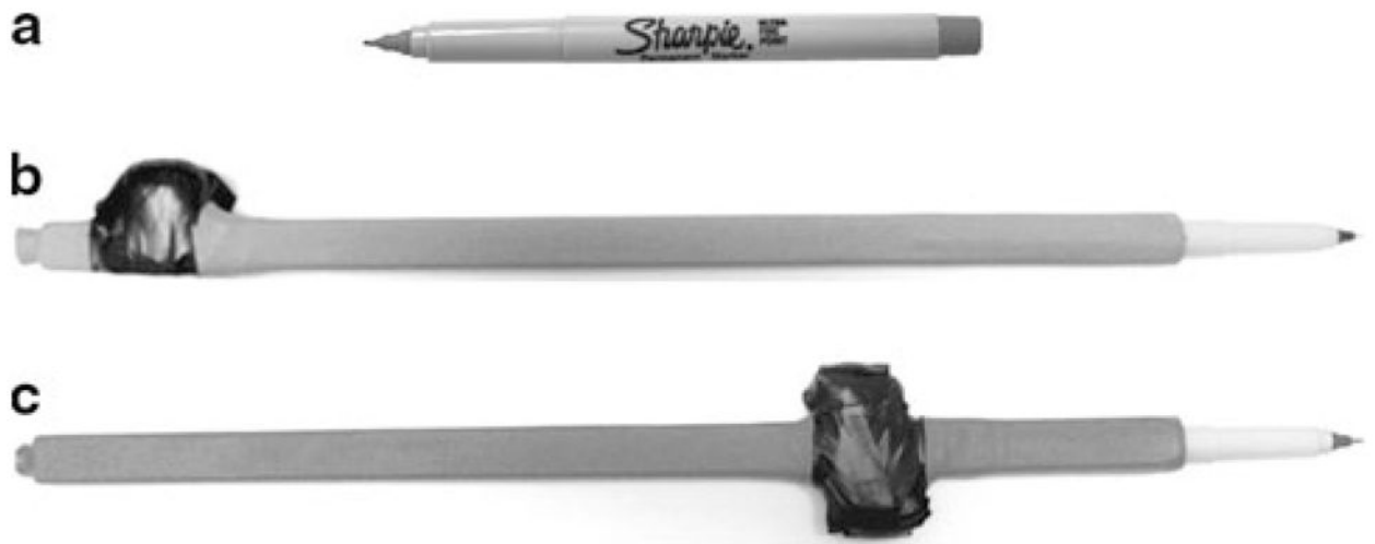
Fig. 1. a Regular pen (non-weighted), b top-heavy tool—with weight positioned at the top, c bottom-heavy tool—with weight positioned at the bottom
