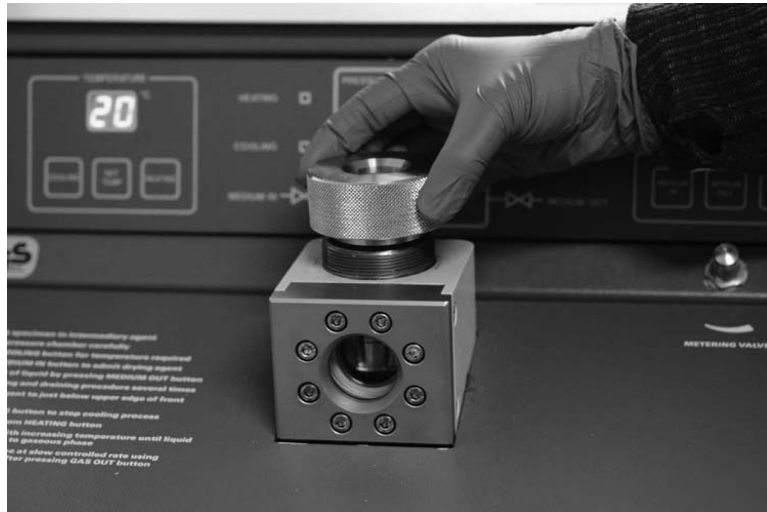
Figure 8. Carefully place the lid on the specimen chamber and make sure it is properly threaded and closed tightly as this chamber reaches high pressure.
