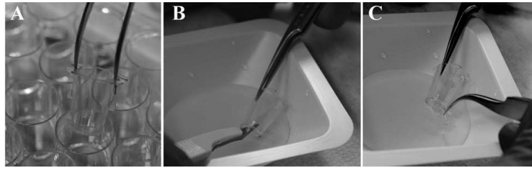
Figure 7. Membrane filter insert removed from 24 cell tissue culture plate (A) is quickly transferred and immersed for trimming in (B) and the membrane is removed with a fine-tipped tweezers (C) for placement in CPD container.
