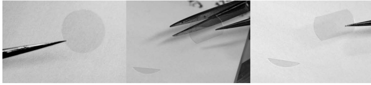
Figure 1. Thermanox™ or aclear materials can easily be trimmed or punched to desired dimensions using a scissors or punch tool for adaptation to size requirements for subsequent processing steps.
