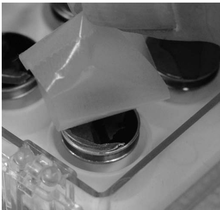
Figure 19. Scotch tape is gently applied to cell layer grown on Thermanox™ coverslips.
