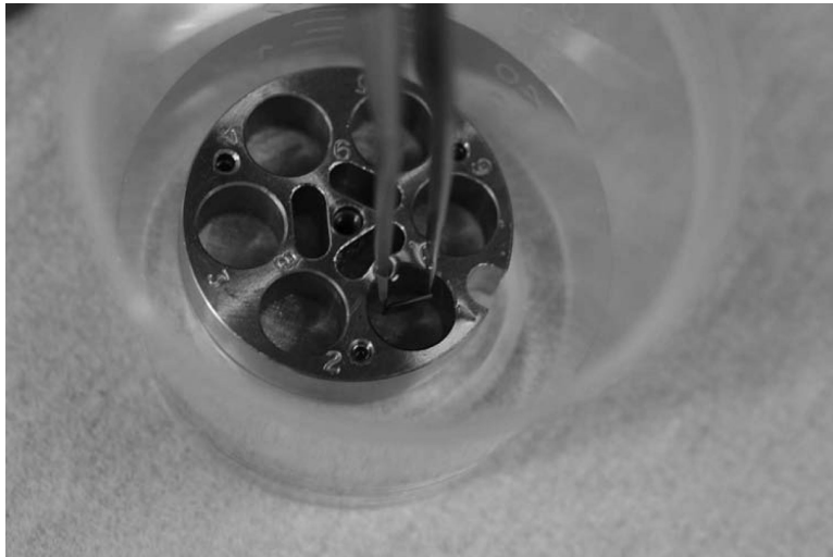
Figure 6. Placement of a chip in specimen vessel used in a Bal-Tec CPD.
