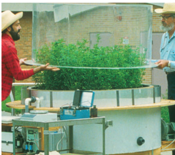
Figure 1 Closing the lid on the photosynthesis chamber. Condensation is visible on ice-cooled lower section.
