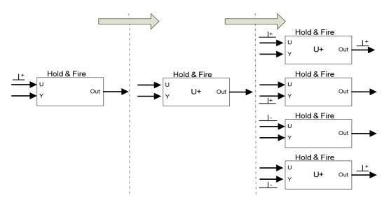
Figure 7. Spikes Hold&Fire evolution form a positive U spike.
