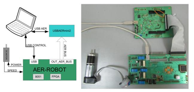
Figure 14. Experimental scenario: (left) block diagram; (right) photography.
