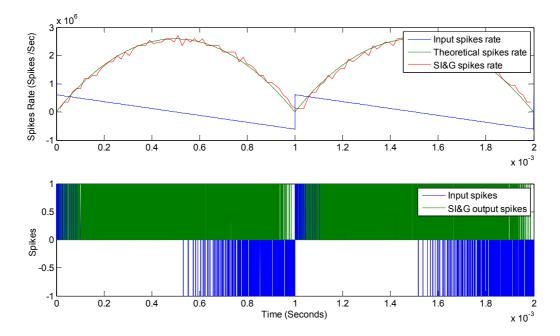
Figure 11. Spikes Integrate & Generate response.
