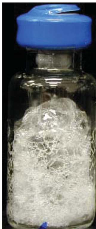
Figure 1. Typical appearance of a foam dried sample. The structure, which occupies a larger volume than a lyophilized cake, is translucent and brittle.
