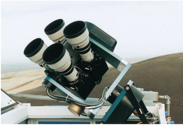
FIG. 2. Four wide-field-of-view ( 17.6 \times 17.6 degrees) cameras of the Livermore Optical Transient Imaging System (LOTIS) (4) survey the sky for OTs from GRBs at a site near Livermore, CA. A similar system, ROTSE (5, 6), operates at a site near Los Alamos, NM.
