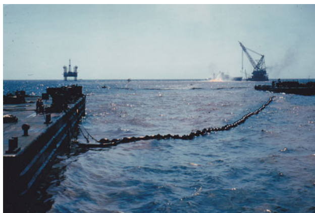
Fig. 2 Ixtoc I, 1979. The booms were not very effective. Oil is shown on both sides of the boom (photograph by Olof Lindén)
