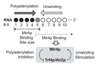
Fig. 6. Coordination between polyadenylation and unwinding activities in TRAMP. O, number of added adenylates;
