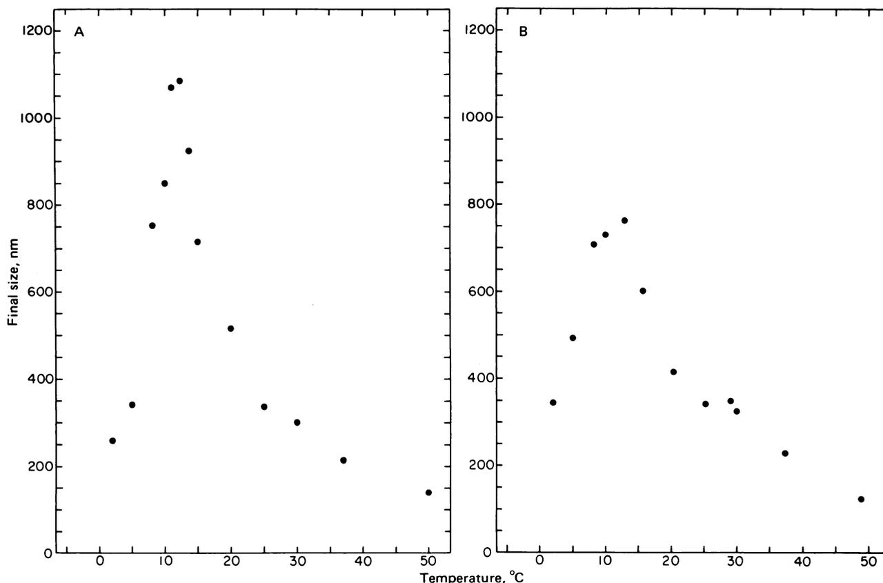
FIG. 2. Final average size as a function of the calcium incubation temperature for two separate preparations (A and B) of sonicated phosphatidylserine vesicles. The final size was measured by using dynamic light scattering after first incubating the sonicated vesicles (<0.5 mM) for, typically, 3 hr in the presence of calcium (<0.9 mM) and then adding EDTA (10 mM).
