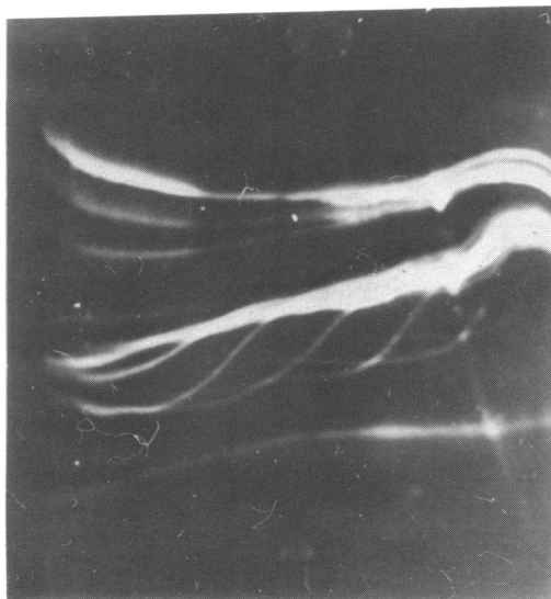
FIGURE 1. Separation of pUC19 DNA topoisomers by denaturing gradient gel electrophoresis. Denaturant concentration increases from left to right. DNA molecules move from top to bottom. The temperature of the gel controlled at 35°C.
