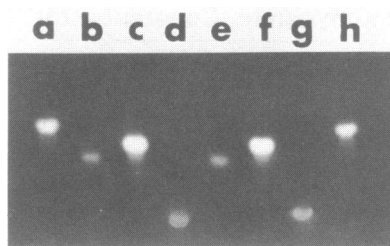
Figure 5. Electrophoresis results in TBM buffer for (a) the Dickerson dodecamer, (b) 1C, (c) 1C·1, (d) 1, (e) 2C, (f) 2C·2, (g) 2, and (h) the Dickerson dodecamer. Because of the weak staining of the oligomers 1 and 2, the bottom of the photograph was exposed for longer than the top to assist in visualization of the fast moving samples. On the gel, their relative intensity is less than for 1C and 2C.
