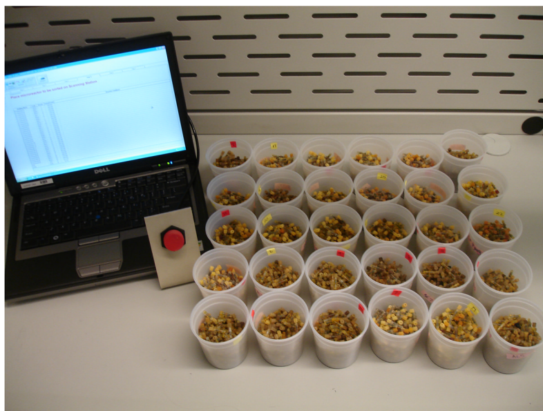
Figure 4. L-Series SynPhase Lanterns equipped with (a) radio frequency (RF) tags and (b) color-coded spindles and cogs. (c) Work station for RF-directed sorting.
