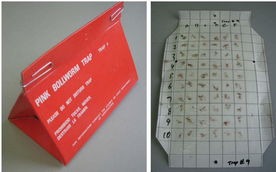
Figure 2. Delta trap: assembled (left) and opened (right) with grids marked A-F horizontally and 1-10 vertically, to hold 60 moths. The inner, white surface is coated with glue, which traps any insects that come into contact with it. doi:10.1371/journal.pone.0038547.g002
