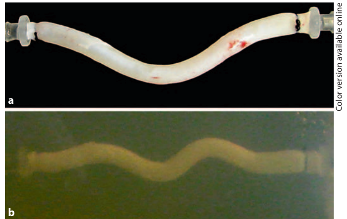
Fig. 5. Photographs of an artery within a supporting matrix under elevated internal pressure buckling into tortuous shapes. a Under an internal pressure (140 mm Hg) beyond its critical pressure (80 mm Hg) in PBS solution. b Under an internal pressure (230 mm Hg) beyond its critical pressure (150 mm Hg) in gelatin. (Photographed by Mr. Shawn Lamm in the author's laboratory).
