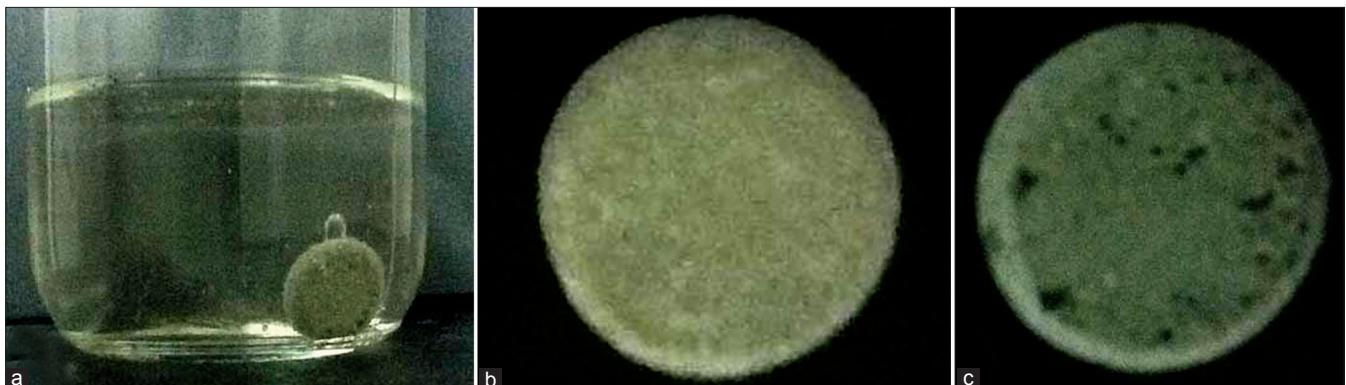
Figure 1: Tablets of aluminium phosphide: (a) in water while releasing phosphine gas, (b) just placed and (c) exposed form (porous feature)
