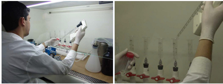
FIG 2 Pipetting of prefiltered sputum digests into 20-ml syringe barrels attached to syringe filter holders loaded with SMFs. The vacuum manifold is made of plastic pipe and valves at a cost of approximately $25. It is connected to a flask, and a vacuum is generated with a hand pump, so no electricity is needed.
