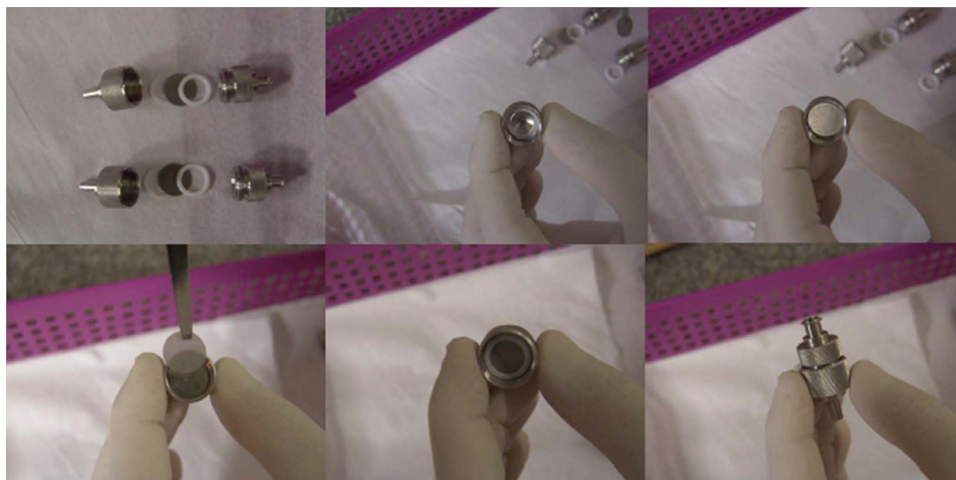
FIG 1 Assembly of small (13-mm) PMFs in stainless steel syringe filter holders.
