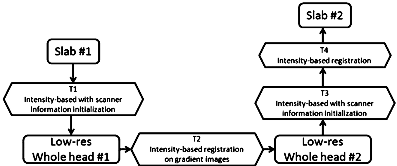
Fig. 6. Overall process used to register slabs acquired during two imaging sessions. All four transformations are computed with an intensity based registration algorithm with NMI as the similarity measure. Transformations 1 and 3 (T1 and T3) use header information retrieved from the scanner for initialization. T2 is computed on the gradient magnitude image of the low-resolution whole head scan. T4 is a simple rigid body transformation as the combination of T1, T2 and T3 is sufficient to bring the images within the capture range of the intensity-based registration.
