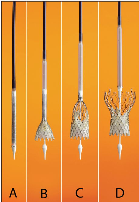
Figure 3. Stepwise desheathing deployment mechanism of Medtronic CoreValve system. A shows the valve completely collapsed within the delivery sheath. B and C show the gradual expansion of the nitinol framed valve as the delivery sheath is slowly retracted. During this stage of deployment, the valve is still attached to the delivery catheter and can be repositioned or even completely recaptured and removed. D shows the final release of the valve from the delivery sheath. With the valve now fully released from the sheath, it can no longer be easily adjusted. (Image provided by Medtronic, Inc. In the U.S., the Medtronic CoreValve® System is available for investigational purposes only.)
