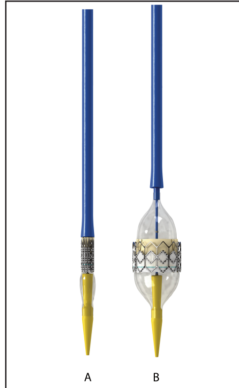
Figure 4. Rapid balloon deployment mechanism of Edwards Sapien system. A shows the crimped valve loaded onto the balloon delivery catheter. B shows the valve being deployed by rapid balloon inflation. With deflation of the balloon, the valve maintains its configuration and the balloon catheter can then be removed leaving behind the fully functioning Sapien Valve. (Published with permission from Edward Lifesciences Inc: Irvine, CA.)
