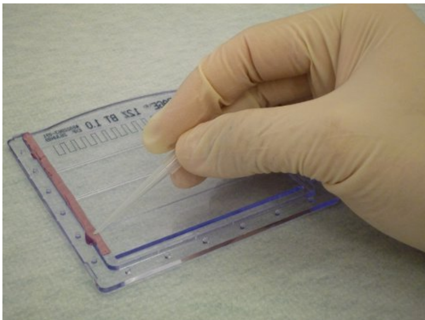
Figure 1. Application of epoxy to seal minigel cassettes. A thin layer of epoxy is applied to the edge of one of the cassettes prior to assembly. To highlight the epoxy, it was false-colored red in this image.
