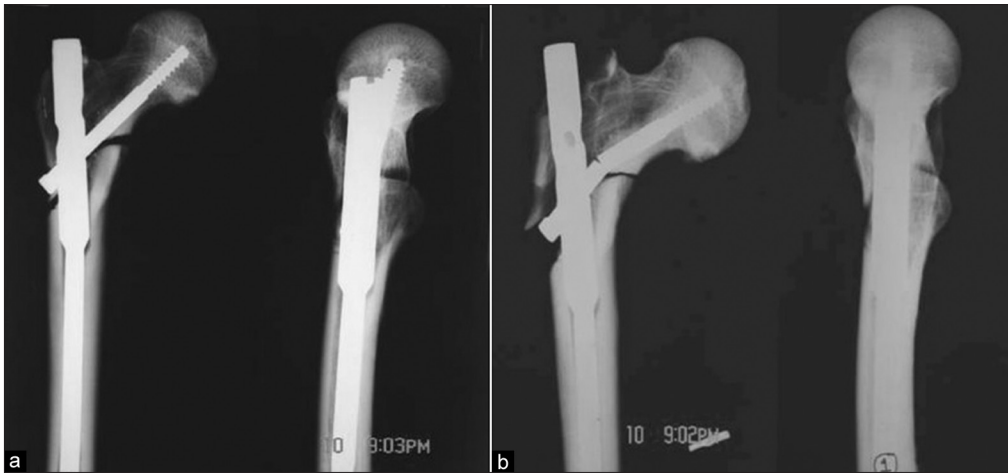
Figure 1: X-rays of cadaveric femoral specimen (a) with unstable reverse oblique trochanteric fracture with posteromedial defect implanted with proximal femoral nail and it was subjected to cyclical compression load. Screw component failed (b) to compression load after 36,000 cycles
