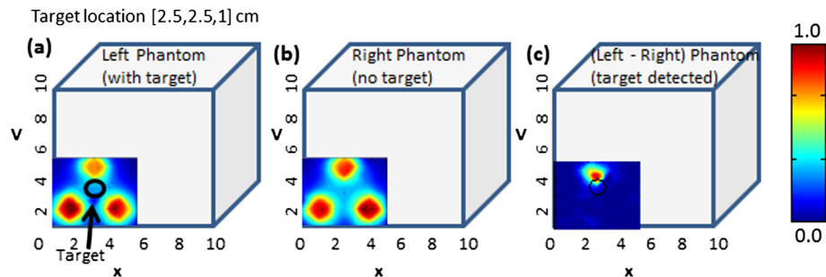
Fig. 8 Two-dimensional surface contour plots of the detected optical intensity in the (a) left phantom with a 0.45 \text{ cm}^3 absorption contrasted target; (b) right phantom with no target. The 10 \times 10 \times 10 \text{ cm}^3 cubical phantom is filled with 1% Liposyn solution and the target is filled with 0.08% India Ink and 1% Liposyn solution. The studies were performed using Gen-2 imager as a simultaneous bilateral imaging (of left and right phantoms) approach. The subtracted (left—right) and calibrated surface contour plot of differential transmission is shown in (c), with the black hollow circle representing the true target location. The contour plots (a) and (b) are normalized individually for better visual representation. The scale of the subtracted contour plot in (c) was converted to a positive scale and further normalized for a distinctly visualizing the improved optical contrast from the unsubtracted image [i.e., (a)].
