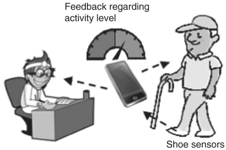
Figure 4. Using the shoe-based sensors to provide behavioral enhancing feedback as part of a telerehabilitation intervention.
