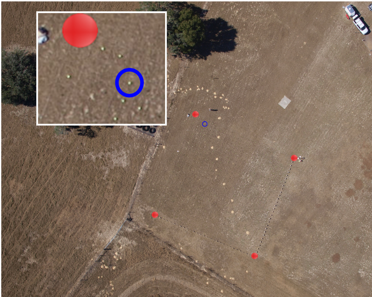
Figure 5. Experimental setup taken from the unmanned aerial system (UAV) at an altitude of 200 m. Red circles indicate the corners of the grid; inset shows a section of the photograph enlarged. Blue circle indicates a tennis ball available for detection. doi:10.1371/journal.pone.0038882.g005
