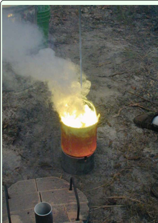
Figure 13. Zinc and zinc slag burn if overheated. The fire can be extinguished by spooning out of the burning material. The chartreuse flame should not be allowed to continue to burn because the fluffy oxides interfere with pouring the zinc. High quality figures and videos are available online.
