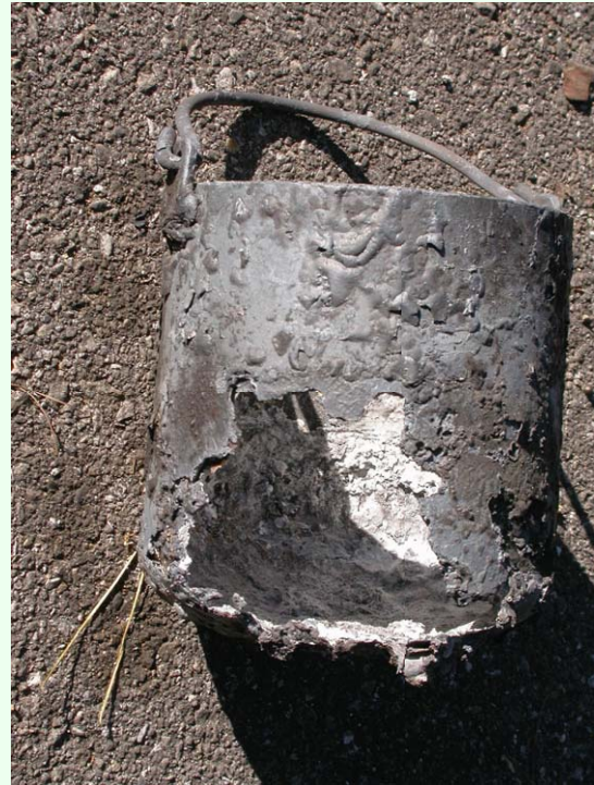
Figure 15. Inattention allowed the kiln to overheat, burning out the crucible and spilling the molten metal into the bottom of the kiln, where it burned a hole and flowed onto the ground underneath. The hole can be seen in Figure 5 (left) but did not affect further operation of the kiln. High quality figures and videos are available online.
