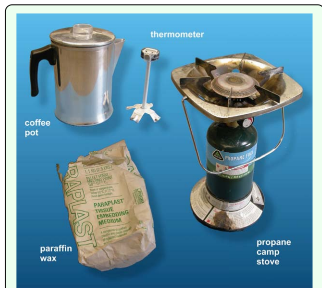
Figure 3. The equipment needed for making nest casts of paraffin wax. The coffeepot makes pouring easy, and the thermometer is needed to prevent overheating of the wax. High quality figures and videos are available online.
