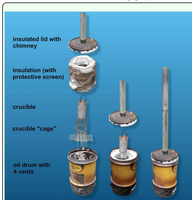
Figure 6. Exploded view showing the construction of the medium, passive-draft kiln. Construction is similar to that of the large kiln, except that 4 air vents were cut at the bottom, and the lid is provided with a tall chimney that creates a draft through the kiln. High quality figures and videos are available online.
