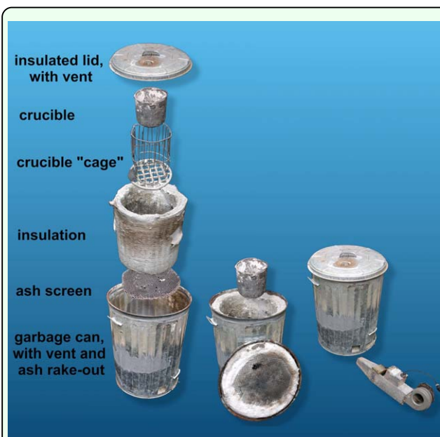
Figure 4. Exploded view of the large forced-draft kiln, showing its parts and their assembly. The air vent at the bottom opens into a space beneath the ash screen, which is supported on a baffle (Figure 5). The insulation and the crucible cage rest on the ash screen, with a space for charcoal between them. Air forced into the bottom rises through the charcoal and is vented through the hole in the insulated lid. High quality figures and videos are available online.
