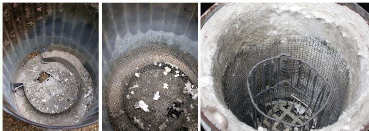
Figure 5. Construction details of the large kiln. (left) The baffle support for the ash screen; (center) the ash screen in place on the baffle; (right) Insulation with its protective screen and the crucible cage in place, ready to receive a load of charcoal and the crucible. High quality figures and videos are available online.
