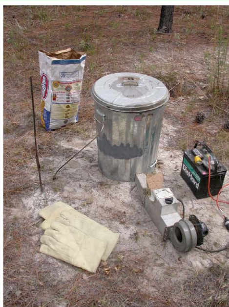
Figure 12. (left) The large kiln in operation. The forced-air draft is provided by a car heater fan powered by a 12-v battery. Stir bar, S-hook, and charcoal are also shown. (right) A crucible containing about 4 L of red-hot aluminum, ready to be poured. High quality figures and videos are available online.
