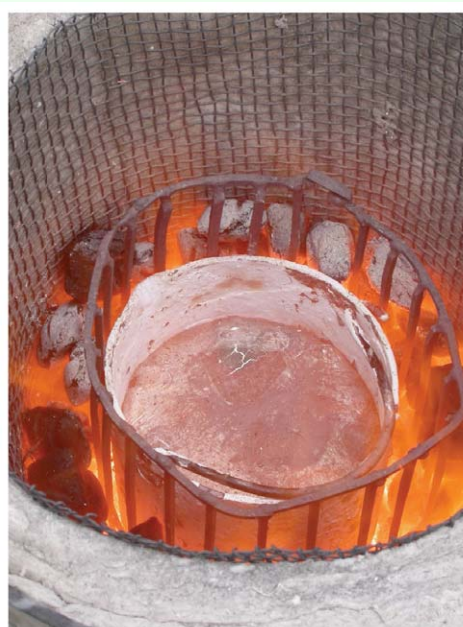
Figure 12. (left) The large kiln in operation. The forced-air draft is provided by a car heater fan powered by a 12-v battery. Stir bar, S-hook, and charcoal are also shown. (right) A crucible containing about 4 L of red-hot aluminum, ready to be poured. High quality figures and videos are available online.
