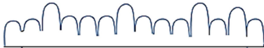
Figure 8. Schematic 2-dimensional profiles for alloy surfaces at different scanning sizes illustrating variation in surface roughness. A) Shows greater variability in surface roughness, with a lower surface area. B) Shows reduced surface roughness variability, with an overall higher surface area due to increased frequency of variation.
