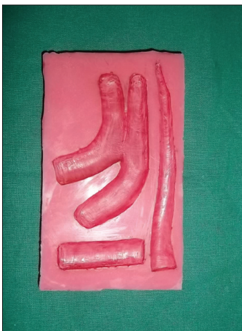
Figure 5: Mould prepared with rapid cure acrylic for making silicon cartilage model
