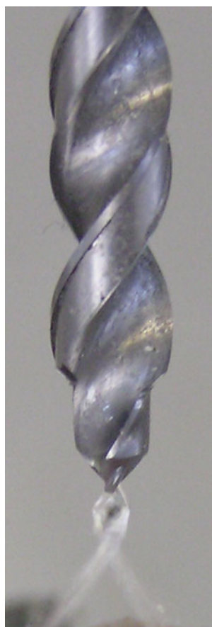
Fig. 3 Two-step drill with diameter of 4.5 mm and channels through the drill with openings on the tip where cooling fluid exits
