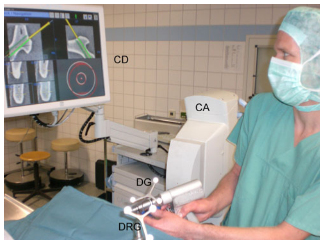
Fig. 1 Operative set-up with the image-guided freehand navigation of the guide wire into the femoral neck using the CAPPa C-Nav navigation system (CAS Innovations/Siemens, Erlangen, Germany). CD image seen on the computer display, DG calibrated guidewire tracker, DRG dynamic reference base, CA C-arm fluoroscope
