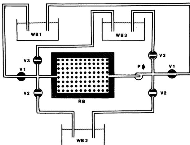
**Figure 2.** Schematic diagram of the automatic temperature-shift apparatus.
