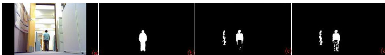
Figure 12. Simulation results for the colour similarity case. (a) Input (b) Ground truth (c) Method: Li et al. ; (d) Method: Zulkifley et al.
