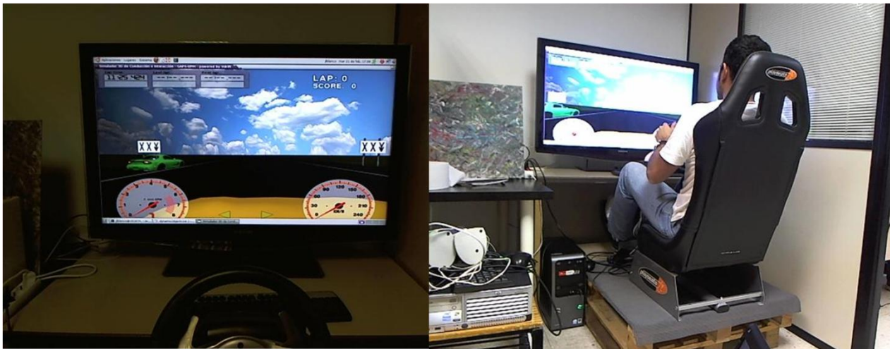
Figure 7. Driving simulator for performance analysis and usability evaluation following the Lane Change Test protocol.
