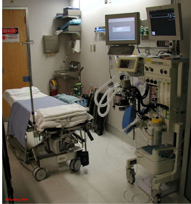
Fig. 2. An AIMS workstation (touch screen and full keyboard), shown mounted on an anesthesia machine (image courtesy W. Sandberg).
