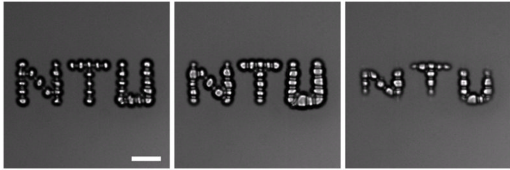
Fig. 3. NTU logo consisting of 34 cavitation bubbles 1.2 \mu\text{s} , 3 \mu\text{s} and 5 \mu\text{s} after the laser pulse ( E=56 \mu\text{J} ). The length of the scale bar is 100 \mu\text{m} .
