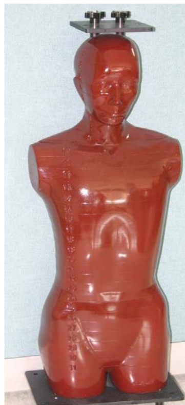
Fig. 1. Alderson radiation therapy phantom.
