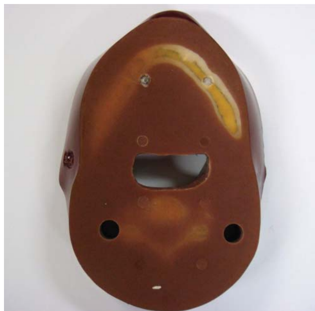
Fig. 2. Thermoluminescent dosimeter (TLD) chips are inserted into each of the organ structures.
