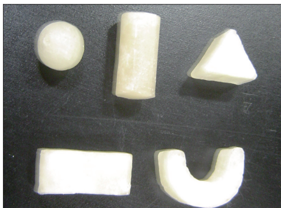
Figure 3. The different shaped wax targets: Sphere, Cylinder, Solid triangle, Dumbbell and U-shaped.
