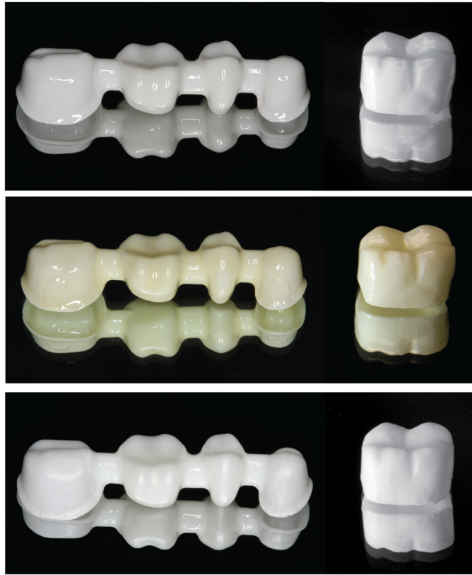
Fig. 10. Graded monolithic glass-zirconia four-unit frameworks and single crowns with white (top) and light yellow (center) shades. Similar framework and crown made from monolithic zirconia (bottom).
