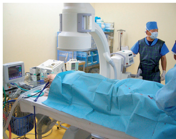
Figure 2 Setting of DSA and operating table for animal (swine) using catheter handling test.
